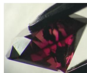
**Figure 5:** A CVD synthetic diamond that has undergone a multistep treatment process to create a Purple-Pink colour. *Photo by Author*
